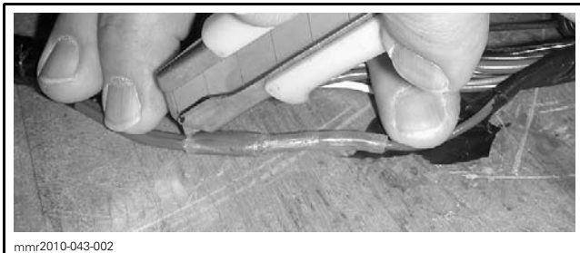
1. Broken wire stripped 2. Splice wire stripped
